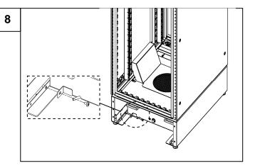
Finally, reinsert the now reversed heat exchanger into the base unit of the LHX 3 and screw the transport securing bracket back in place (Figs. 7 and 8).
