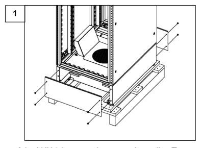
At delivery the base of the LHX 3 is secured to a wooden pallet. To remove this, first unscrew the covers to front and rear of the LHX 3 (Fig. 1).
