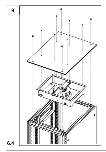
Caution! While removing or working on the fan unit please first remove the mains plug from the power supply (see safety regulations, page 5).
