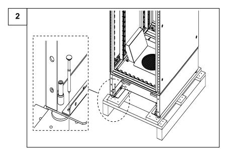
Now simply unscrew the retention screws between the cabinet base and pallet (Fig. 2).
